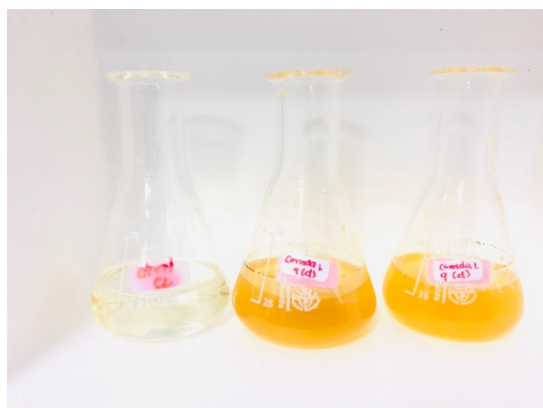
Figure 30 A) Run # 1 of the Box-Behnken experimental design at operating conditions: Temperature 30, incubation time nine days, and agitation 100 rpm; reporting the highest concentration (445 \mu\text{g/mL} ). B) Run #13 of the experimental design, operating conditions: Temperature 35, incubation time five days, and agitation 150 rpm; reporting the lowest concentration (17.5 \mu\text{g/mL} ). Each run was inoculated with the same biomass (30 mg). The control of each test was performed without inoculum and under the same concentrations of the corresponding runs.
