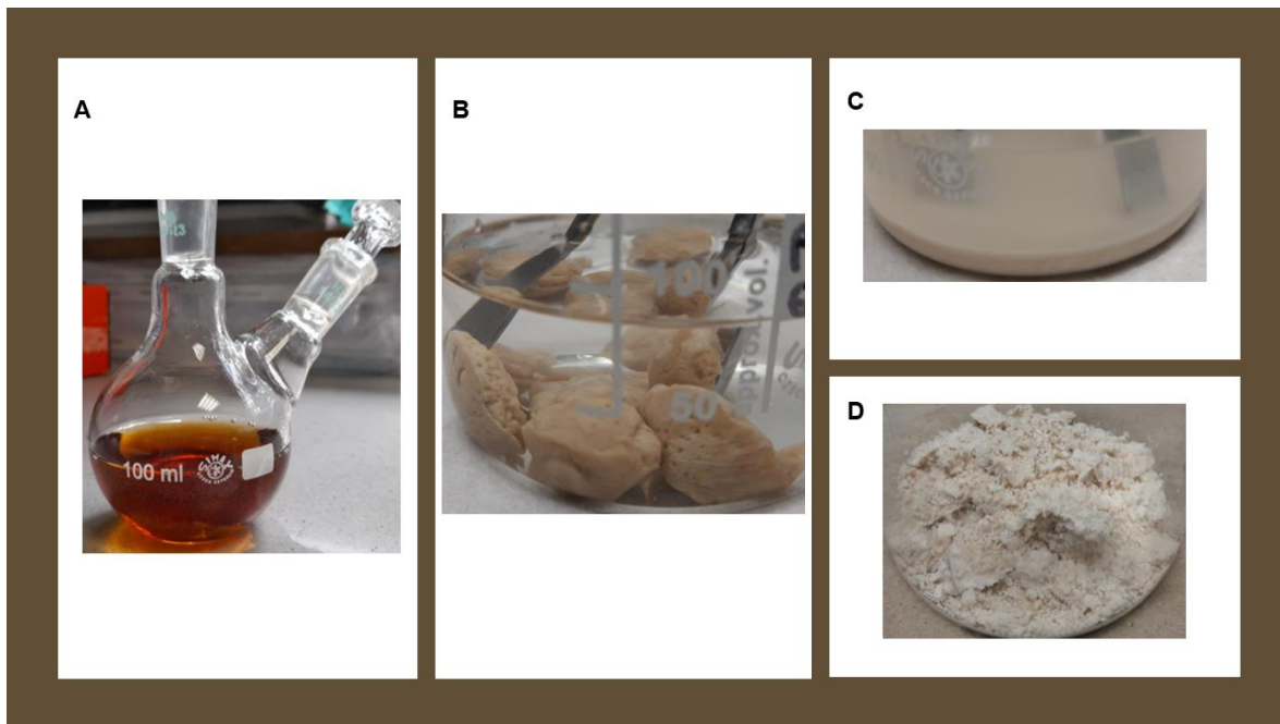
Figure A 1. Synthesis of zwitterionic starch after (A) twelve-hour of reaction, (B) neutralization, precipitation, and three wash with methanol, (C) smash in methanol, and (D) filtration.
