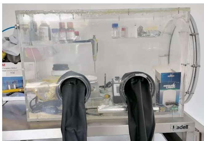
Figure 20. Operating glove box. Three shelves were added to the glove box to organize reactants, samples, and instrumentation. The blue hose of the left enables nitrogen flow; the yellow hose allows pump extraction.
