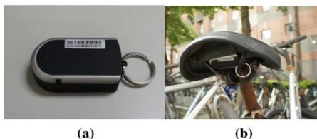
**Figure 2 (a) the Bluetooth device (b) mounted to a bicycle. We used a keychain and double-sided tape to lock the tag underneath the Bike**
