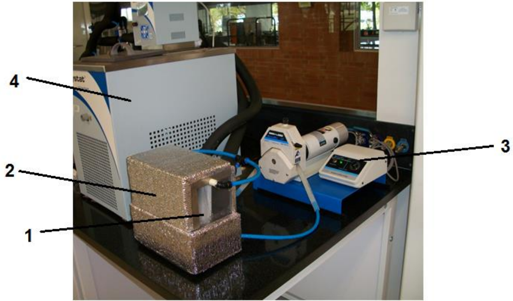
Figure 2.8. Falling-film freeze concentrator.
