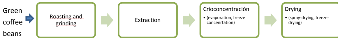
Figure 1.1. Process used to obtain soluble coffee
