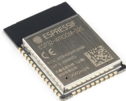
Figura 17. “Microcontrolador ESP32 WROOM - 32E” (Espressif Systems, 2022)
